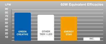
At 81 LPW, this lamp's efficacy is higher than the Tier 1 LED BR30 65W replacement industry average and exceeds the new ENERGY STAR 2.0 requirements. This energy-saving performance makes this lamp a smart retrofit choice for incandescent bulbs.
