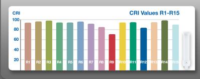
THE CRI<sup>SP</sup> SERIES PL H 10.5W lamp features a typical CRI 90, R9 66 and R13 96, providing crisp and vibrant colors across the whole spectrum. Its exceptional R9-R14 values (R9 & R13) provide redder reds, natural looking skin tones and whiter whites.
