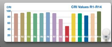
The CRI<sup>SP</sup> SERIES A21 15W lamp features a typical CRI 90, R9 50 and R13 90, providing crisp and vibrant colors across the whole spectrum. Its exceptional R9-R14 values (R9 & R13) provide redder reds, natural looking skin tones and whiter whites.
