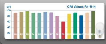
The CRI<sup>SP</sup> SERIES A21 18.5W lamp features a typical CRI 90, R9 60 and R13 90, providing crisp and vibrant colors across the whole spectrum. Its exceptional R9-R14 values (R9 & R13) provide redder reds, natural looking skin tones and whiter whites.
