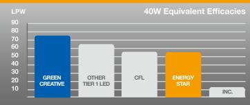
At 75 LPW, this lamp's efficacy is over 10% higher than the Tier 1 LED A19 40W replacement average and exceeds the new ENERGY STAR requirements by upwards of 35%. This energysaving performance makes this lamp a smart retrofit choice for incandescent and CFL bulbs.
