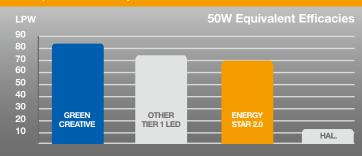
At 83 LPW, this lamp's efficacy is higher than the Tier 1 LED GU10 50W replacement industry average and exceeds ENERGY STAR 2.0 requirements. This energy-saving performance makes this lamp a smart retrofit choice for halogen bulbs.
