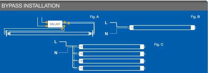
J Bypass ballast by cutting all wires as in Fig. A
