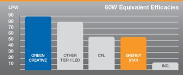
At 89 LPW, this lamp's efficacy is more than 10% higher than the Tier 1 LED A19 60W replacement industry average and exceeds new ENERGY STAR requirements by upwards of 62%. This energysaving performance makes this lamp a smart retrofit choice for incandescent and CFL bulbs.
